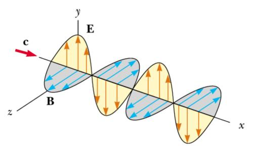
An EM wave **linearly** polarized in the y direction
