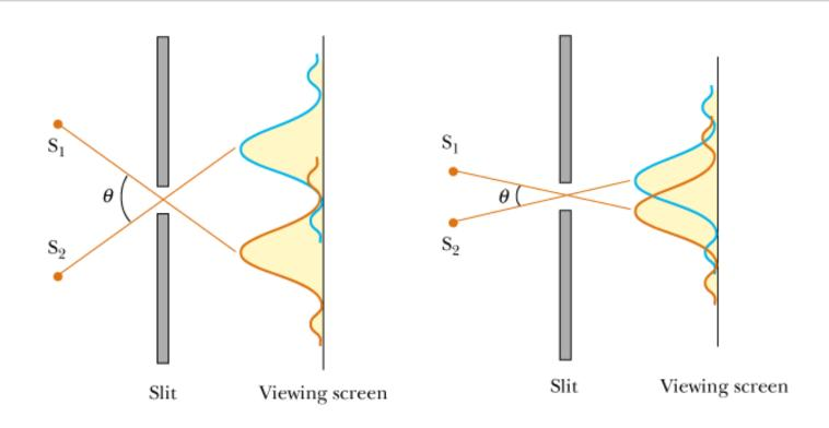
When the central maximum of one image falls on the first minimum of the other Image, the images are said to be just resolved. This limiting condition is called the **Rayleigh's Criterion**.
